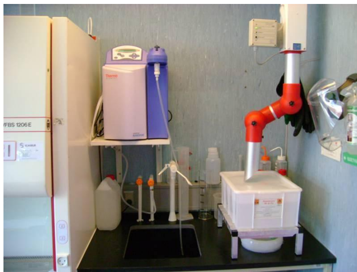
Figure 1. Example of Thermo Nanopure Diamond® UV-water system (Thermo Scientific).
