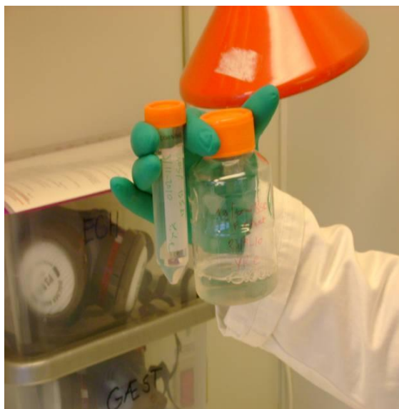
Figure 3. Flask with raw 1% w/v BSA solution and a 1% w/v sterile-filtered BSA-solution in a centrifuge vial. After sterile filtration the 1% w/v BSA stock solution can be kept in a refrigerator for at least 2 weeks.
